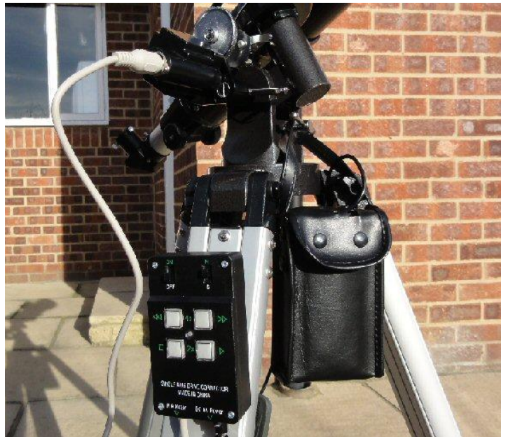
The RA Drive Motor, Control Box and Battery Pack fitted
