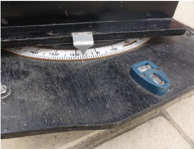
The Azimuth Bezel on the Dobsonian Telescope
