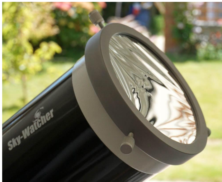
Mylar Solar Filter fitted to a Reflecting telescope
