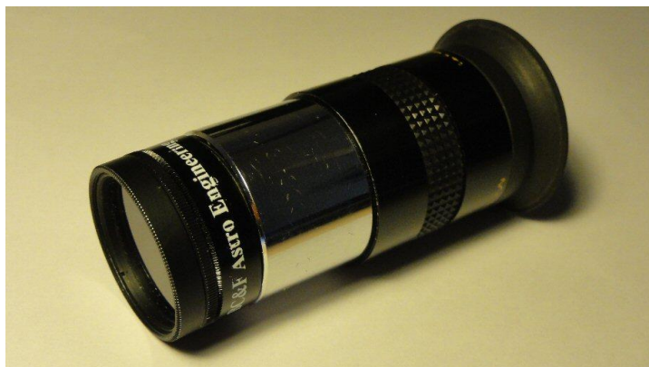
A Polaroid Moon Filter fitted to an eyepiece
