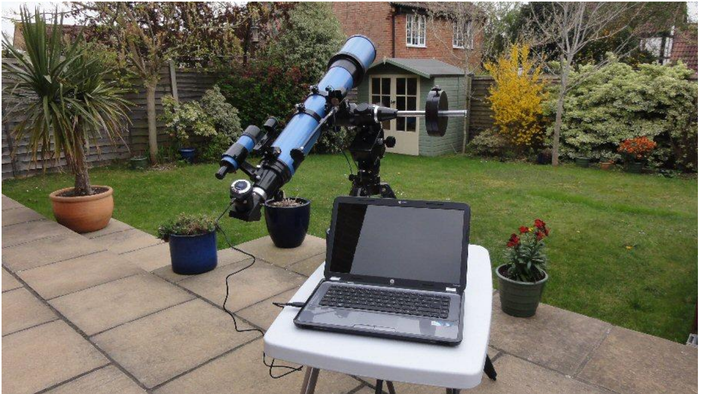
The image above shows a webcam fitted to a 120mm Skywatcher refracting telescope
