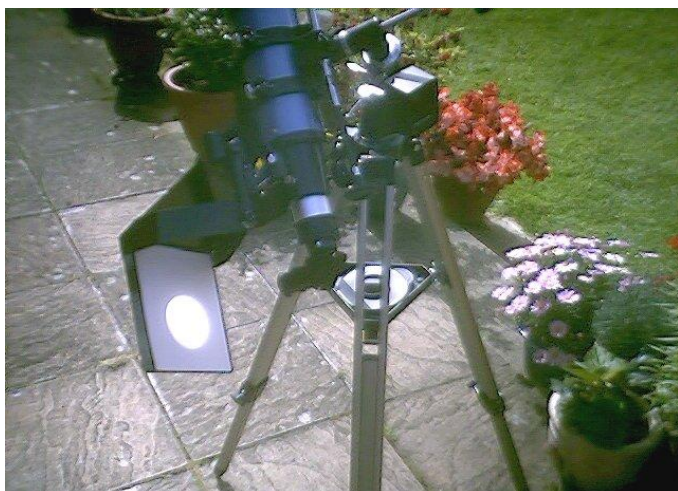
A Solar Observing Screen attached to a telescope
