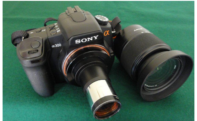
A DSLR with a focuser adapter fitted
