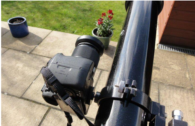
A DSLR 'piggy backed' on a telescope mount
