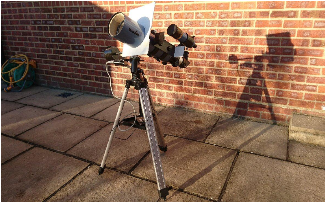
The author's 102mm by 400mm f l Skywatcher refractor adapted for solar observing
