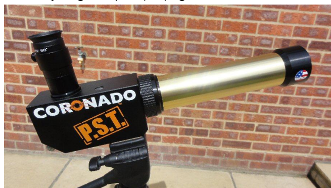
A Personal Solar Telescope (PST) H\alpha telescope Approximate purchase price £800.
