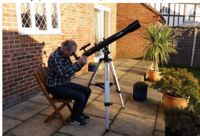
The author's 90mm x 900mm focal length telescope
