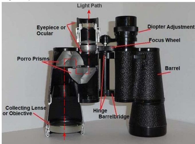
The typical light path through a binocular
