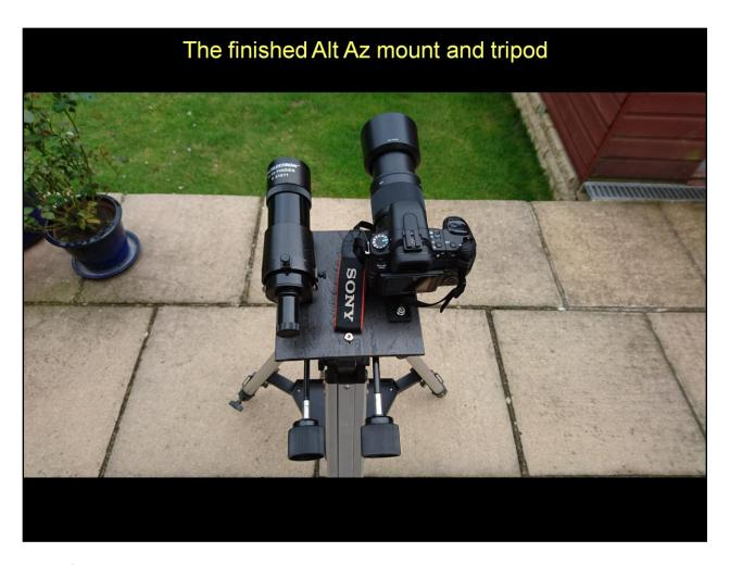
The finished assembly showing the Alt Az mounting movement knobs.
