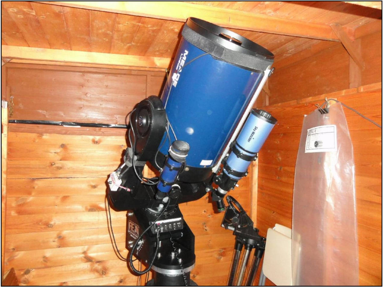
The telescope in the polar alignment position. Pointing to the Celestial Pole 90^\circ Dec.
