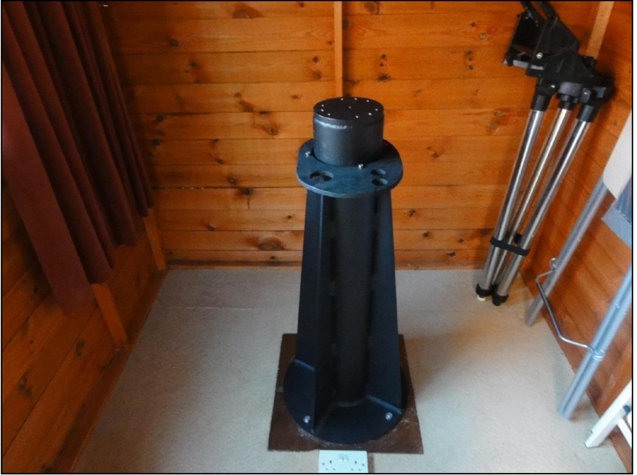
The pier in position and secured to the mount.
