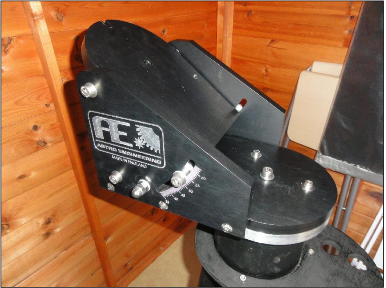
A close up view of the wedge latitude angle setting mechanism.
