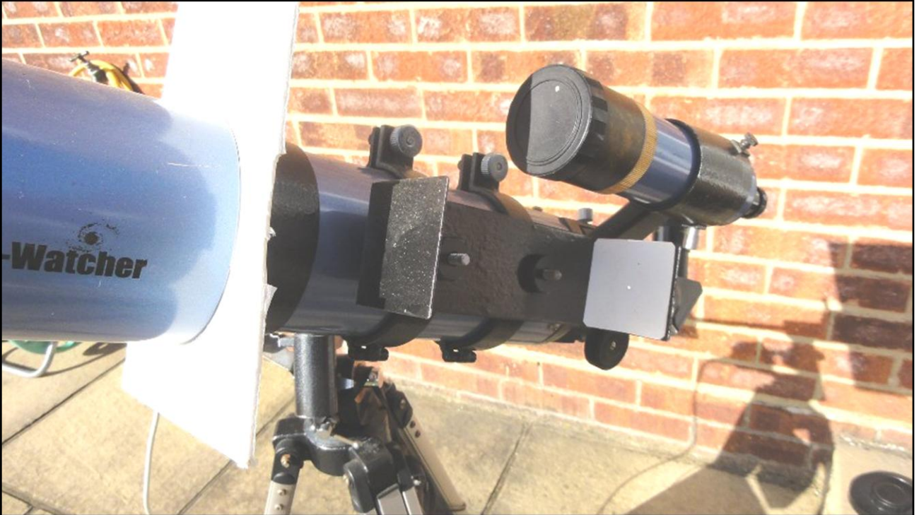
Front screen with pin hole and back screen a white card
